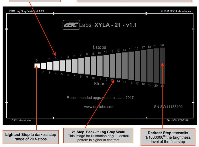
Xyla 21 darkest step transmits 1/1000000<sup>th</sup> the brightness level of the first step, so to be meaningful all readings should be taken in a darkened room. Xyla also features sliding shutters that enable individual steps or groups to be isolated to reduce the dynamic range; this can also identify flare in camera lenses and other optical elements.
