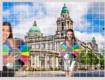
4) Insert number of horizontal squares covered by ChromaDisk into table; in this case, three squares. Similarly, enter the maximum visible resolution, here "F", into table). This shows that the camera resolution is 1143 pixel width.
