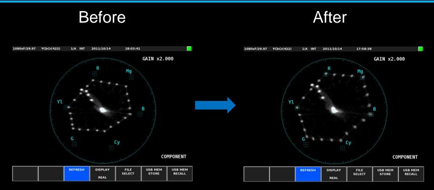
Adjust the Linear Matrix controls and try to put the colors vectors in their boxes.
