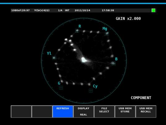
Once you get close to the color targets using the Linear Matrix, you can then fine tune (polish) using the Color Correction. Note, avoid using too much phase control, if you see the dots on the vectors scope become oblong you are creating noise. Go very gentle and don't worry if you cannot reach a given color target. The end result will still look great, but without adding noise!
